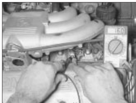
20.5 Check the resistance of each of the fuel injectors
