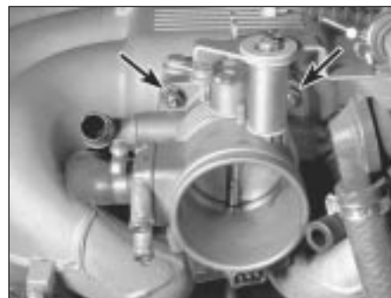
17.11 Remove the nuts (arrowed) and lift the throttle body from the intake manifold (the two lower bolts are hidden from view)
