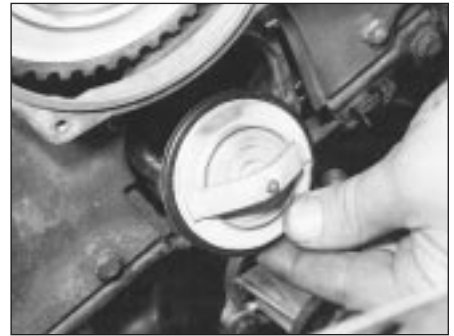
3.20b Removing the thermostat (M40 engine)
