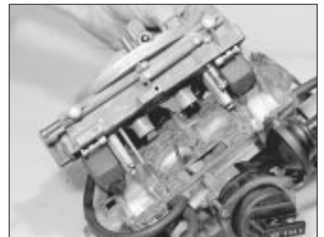
12.6a Lifting the cover from the carburettor main body
