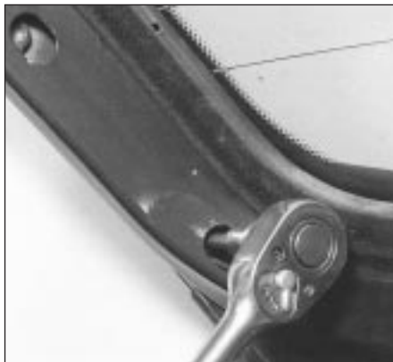
14.14 Unscrewing the hinge mounting bolts (5-Series)
