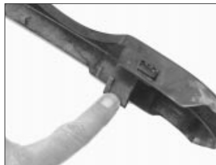
9.10 Detach the centre grille valance by reaching under each headlight and pressing on the release lever
