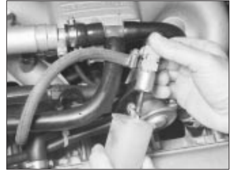
19.2 Watch for a steady, conical-shaped spray of fuel when the starter motor is operated
