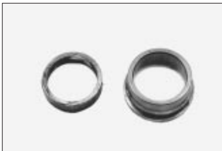
15.14b You can fabricate your own spacer tool from a piece of 13 mm long, 38 mm inside diameter pipe (left); you'll also need to use the old inner race (right)
