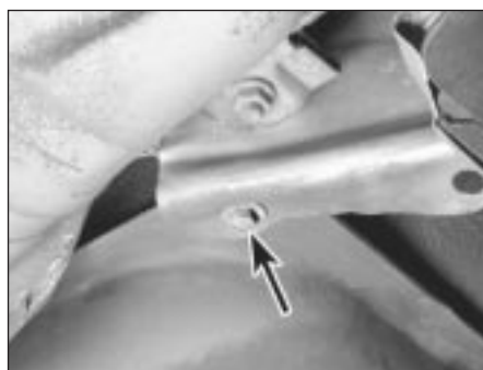
6.10a Remove the fuel tank mounting bolts (one arrowed)
