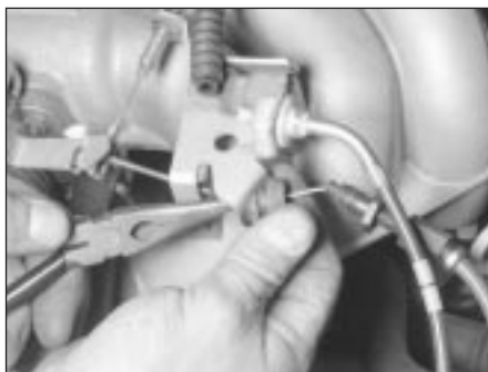
9.8 Push the rubber grommet from the rear, and separate the cable from the bracket
