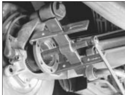
15.11 Remove the drive flange with a puller
