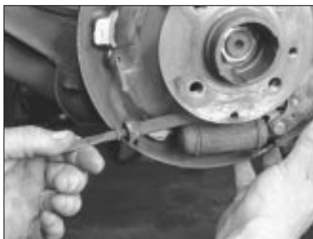
6.8 Remove the automatic adjuster assembly
