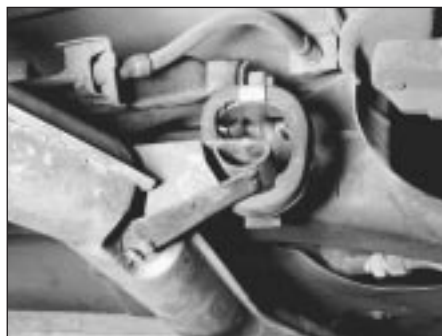
22.1 A typical exhaust system rubber mounting
