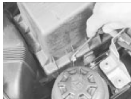
20.5 Use a screwdriver to detach the air cleaner cover clips
