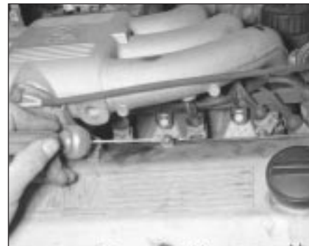
15.7 Use a stethoscope or screwdriver to determine if the injectors are working properly - they should make a steady clicking sound that rises and falls with engine speed changes
