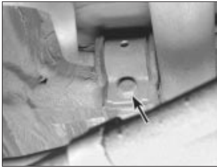
12.2 Rear anti-roll bar bracket bolt (arrowed) (3-Series)
