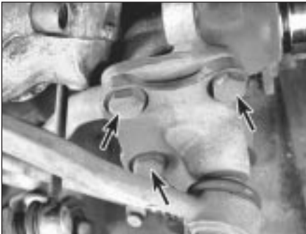
4.5 If you're removing the control arm, remove the three bolts (arrowed) from the steering arm, and separate the strut assembly from the arm
