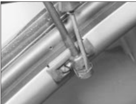
14.12a Removing the tailgate strut spring clip (3-Series)
