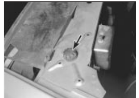
10.19 Screw the bonnet stops in or out after making other adjustments
