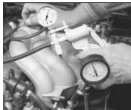
18.5 Carefully watch the fuel pressure gauge as vacuum is applied (fuel pressure should decrease as vacuum increases)
