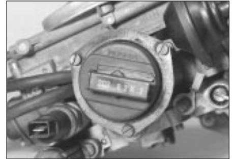
12.17 Remove the three screws and withdraw the metal ring
