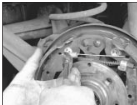
6.5a Unhook the upper return spring from the front shoe . . .
