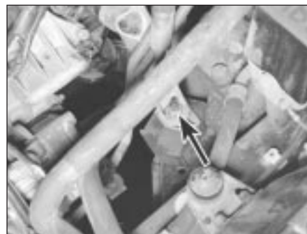
17.10 To remove an engine mounting, first remove the stud nut (arrowed) - M30 engine shown, others similar
