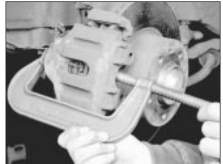
3.5i Depress the piston with a C-clamp (5-Series)
