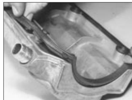
4.7c Removing the valve cover gasket on the M40 engine
