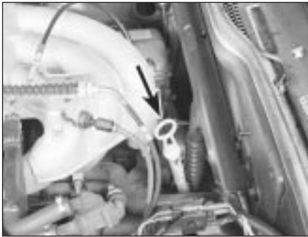
8.5 The automatic transmission fluid dipstick (arrowed) is located near the bulkhead on the left side of the engine compartment
