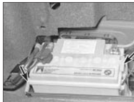
3.3a Always detach the cable from the battery negative terminal first, then detach the positive cable - to remove the hold-down assembly, remove the nuts (arrowed) or single bolt
