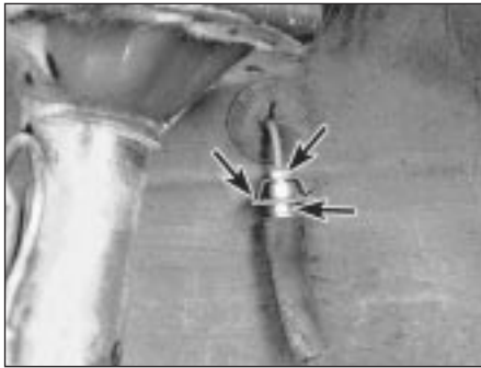
15.3 A typical brake line-to-brake hose connection: To disconnect it, use one spanner to hold the hex-shaped fitting on the end of the flexible hose (lower right arrow) and loosen the threaded fitting on the metal line with a split ring ("brake") spanner (upper right arrow), then remove the spring clip (left arrow)
