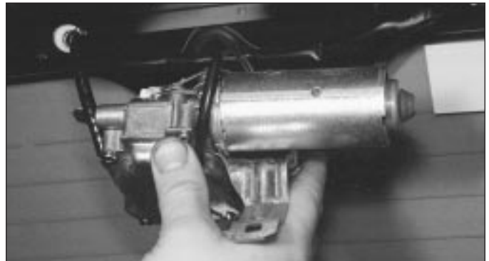
16.11a Removing the tailgate wiper motor (3-Series)
