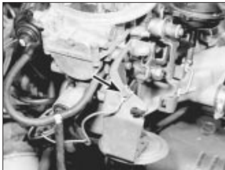
11.5 Remove the screw, and disconnect the carburettor earth cable (arrowed)
