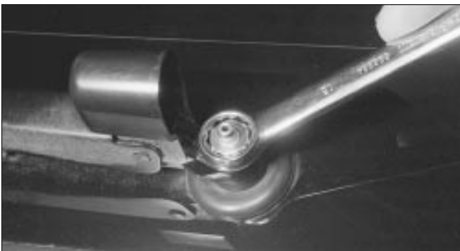
16.9 Removing the tailgate wiper arm nut (3-Series)
