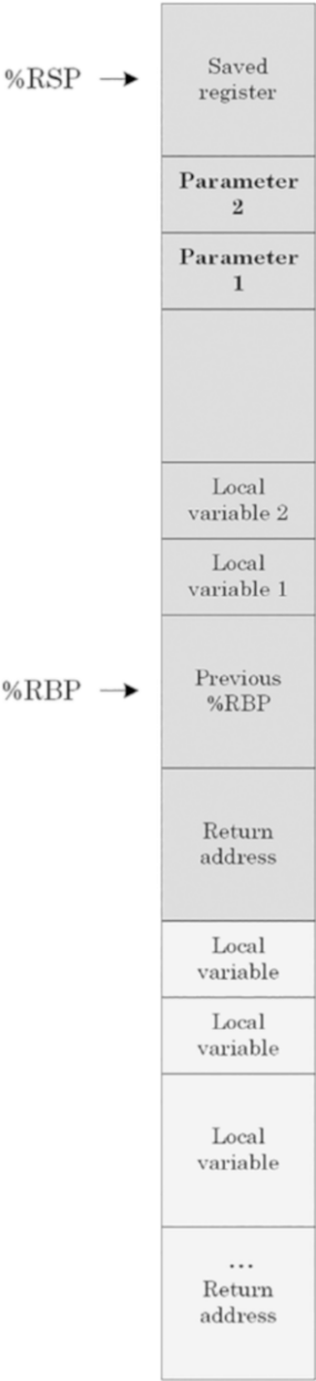
Figure 11-1. Stack memory layout for the function with two arguments and two local variables
