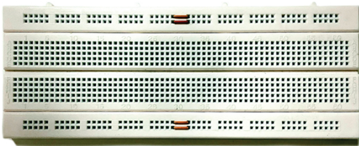
Figure 10-1: Notice the jumper wires to extend the power rails along the entire length of the breadboard.
