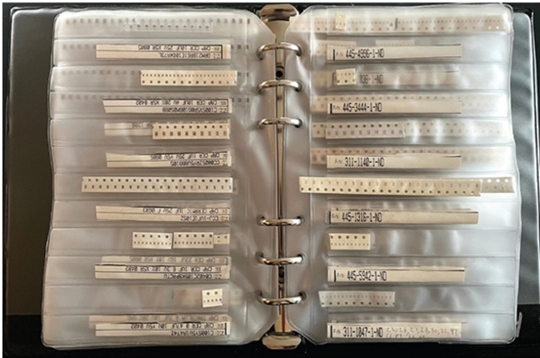
Figure 11-3: A binder for holding cut tape
