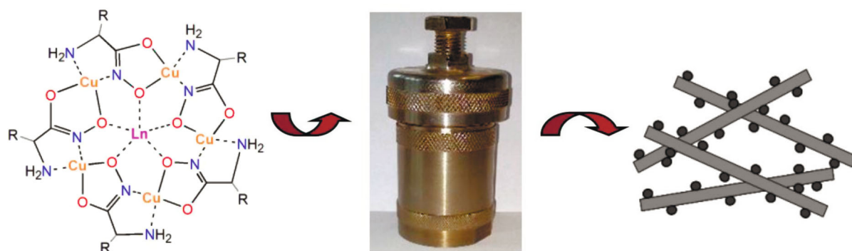
Fig. 16. Scheme of the hydrothermal synthesis of hybrid materials based on metallacrowns and MWCNTs.
