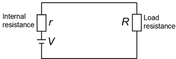
Fig. 4.5 Circuit in which the load resistance R and internal resistance r at the power supply are connected
