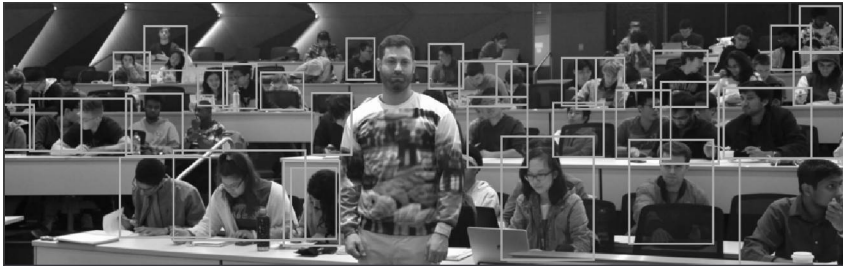
Image 15-1: A “stealth” adversarial pattern on clothing causes object detectors (e.g. YOLOv2) to ignore the wearer [23]. In this demo, every other person (blue boxes) is detected except the man in the adversarial sweater. The patch’s colorful design was optimized so the detector’s “person” confidence stays low, effectively rendering the wearer invisible to the model [1].
