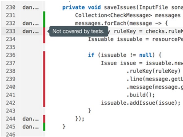
Figure 8-12. Many static analysis tools like SonarQube also show line-level coverage results
