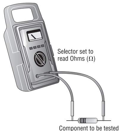
FIGURE 13.11 Connecting a multimeter to measure resistance
