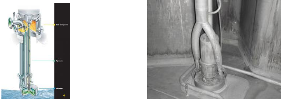
Figure 2: Deepwell cargo pumps.
