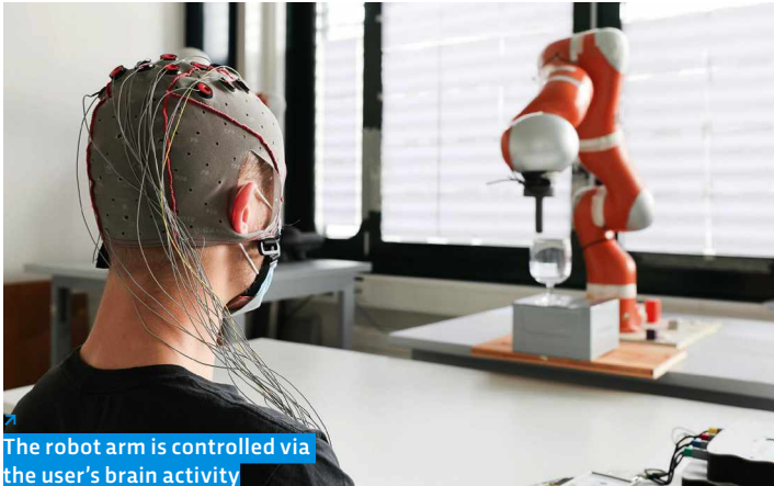
The algorithm reads the user's brain for feedback on how the robot is moving
