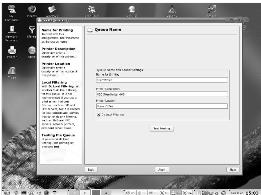
Figure 18-11: Setting queue values for an SMB printer in YaST
