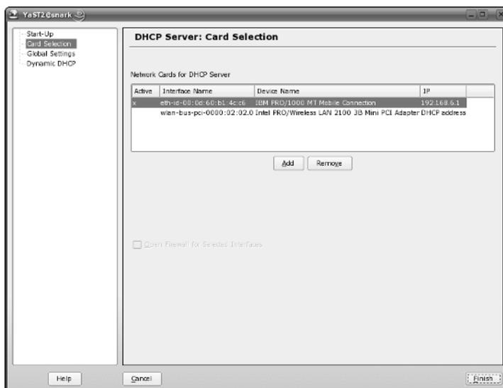
**Figure 20-6:** The DHCP Server configuration editor's Card Selection screen
