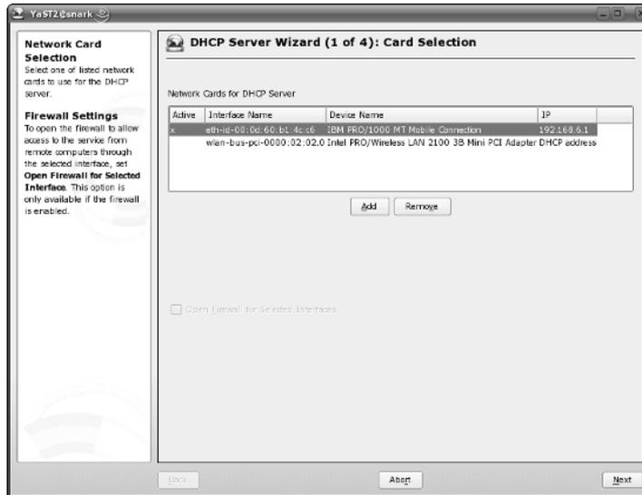
**Figure 20-1:** The Card Selection screen of the YaST DHCP Server Wizard
