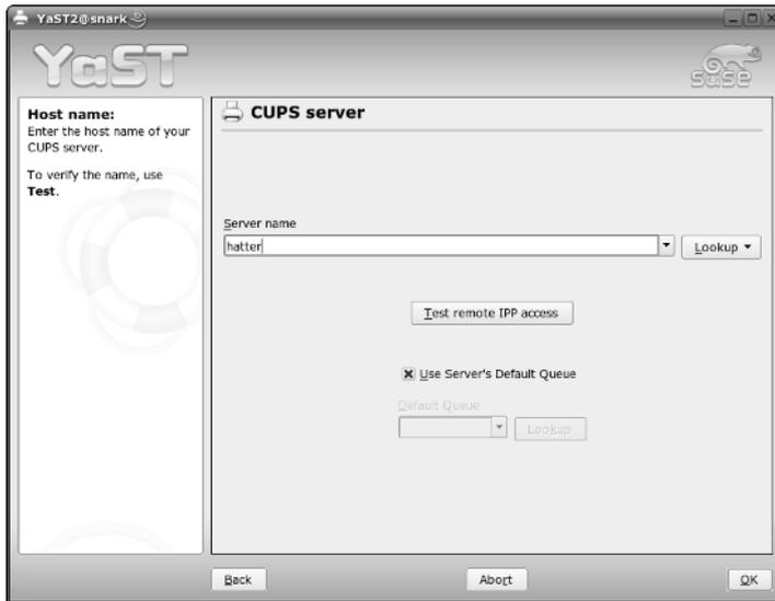
Figure 19-6: Setting up the remote CUPS server in YaST
