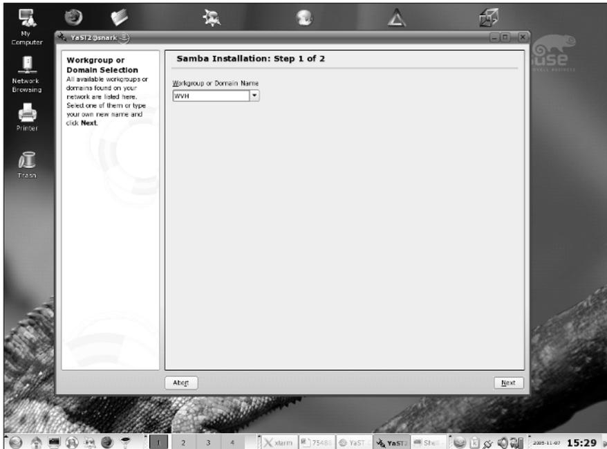
Figure 18-13: Initial Samba Server configuration screen in YaST
