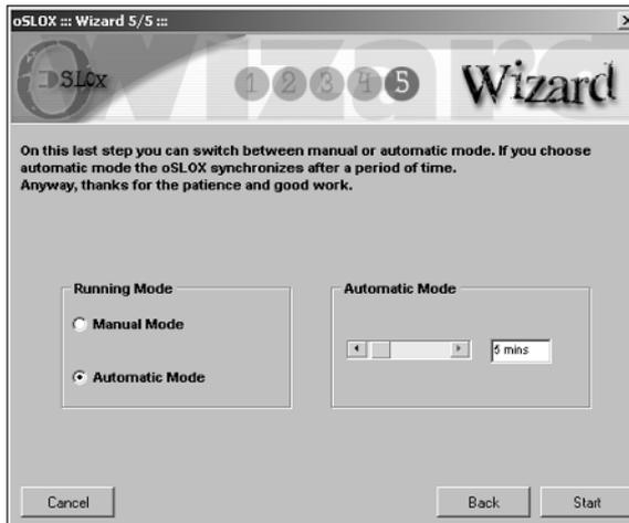
**Figure 30-40:** Configuring synchronization time
