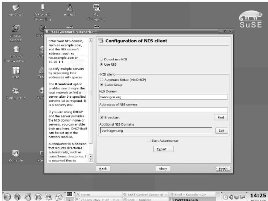
Figure 22-7: Configuring an NIS client in YaST
