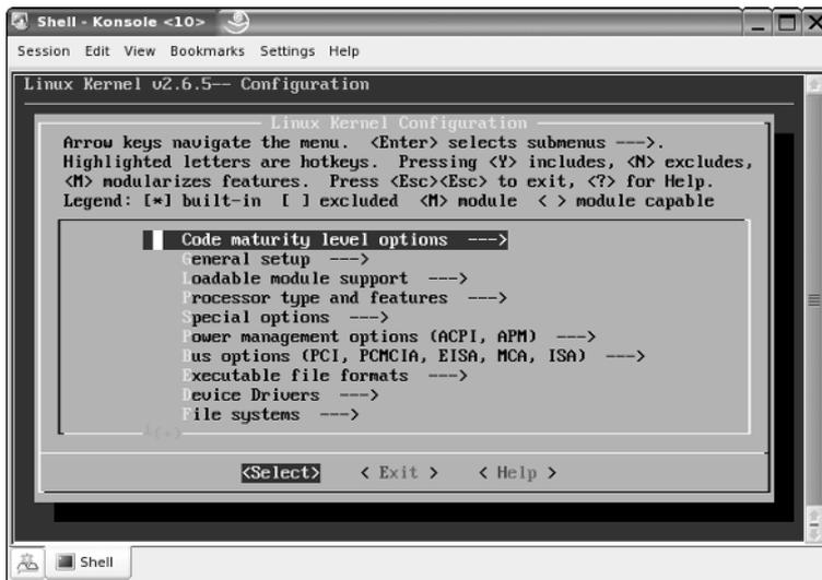
**Figure 29-1:** Using `make menuconfig` for kernel configuration
