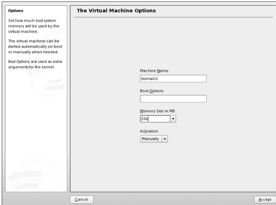
**Figure 28-8:** Setting Xen virtual machine options in YaST
