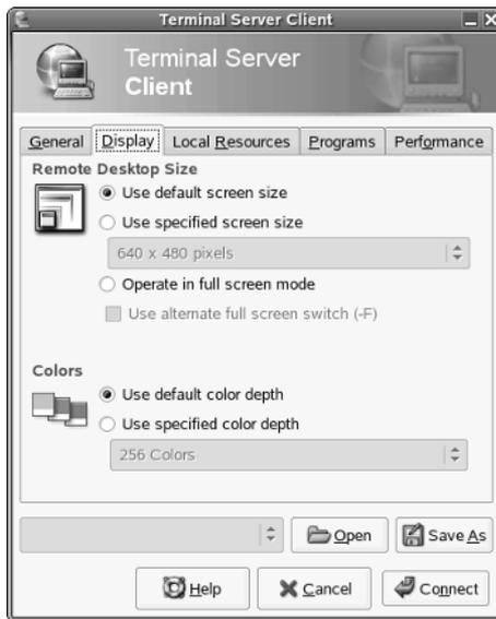
Figure 32-4: The Terminal Server client connection dialog box
