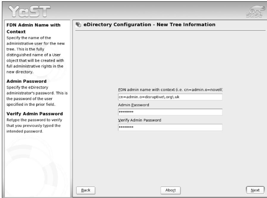
**Figure 31-7:** The eDirectory configuration during the installation of OES
