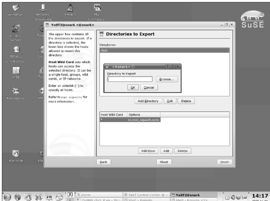
Figure 22-2: Configuring the NFS server with YaST
