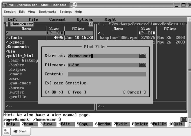
Figure 13-3: Finding files with mc
