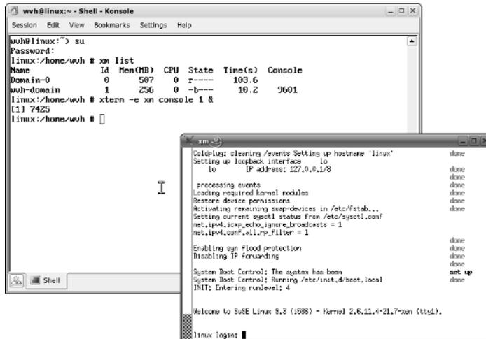
**Figure 28-12:** A console prompt for a Xen virtual machine
