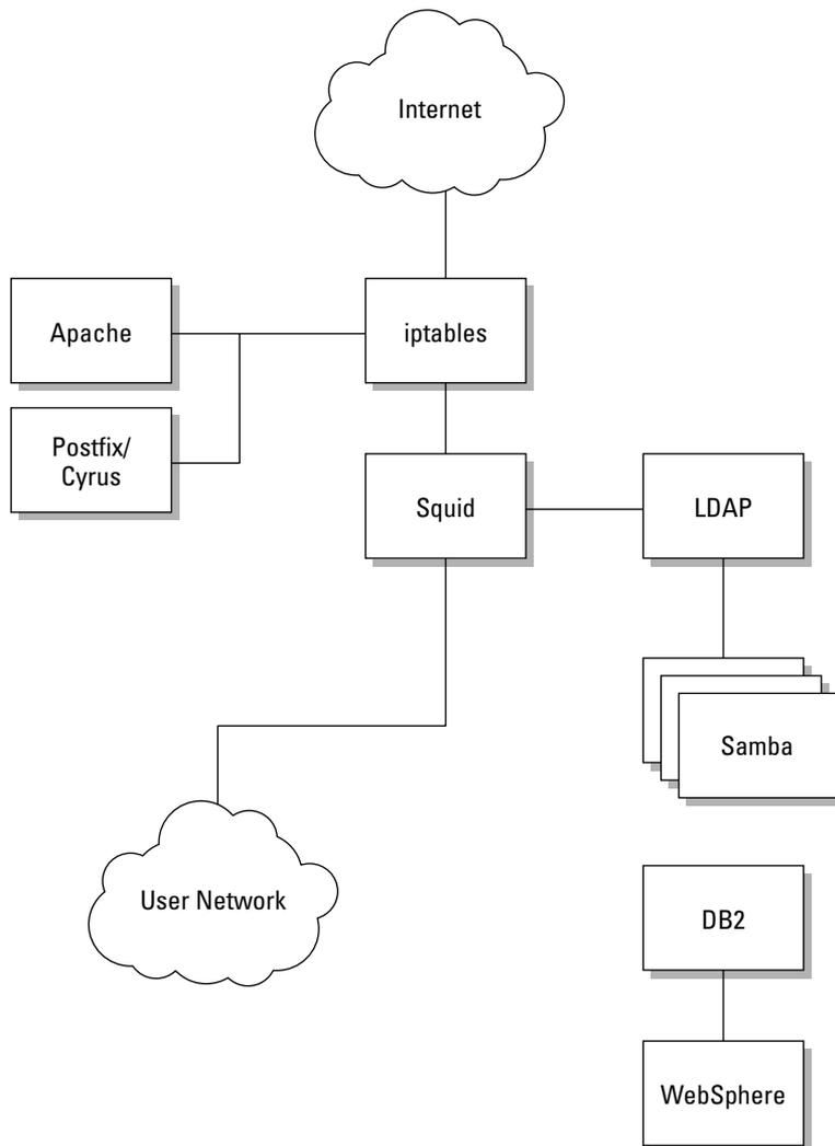
**Figure 27-3:** Linux implementations of the generic network components
