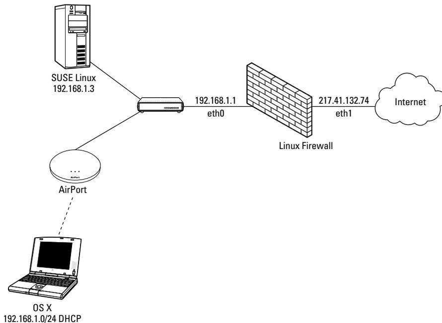
**Figure 24-2:** Network using a netfilter firewall
