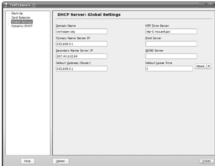
**Figure 20-7:** The DHCP Server configuration editor's Global Settings screen
