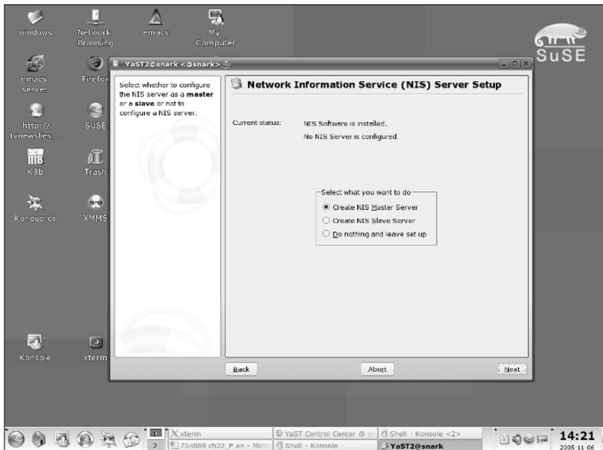
Figure 22-3: The YaST module for NIS Server configuration
