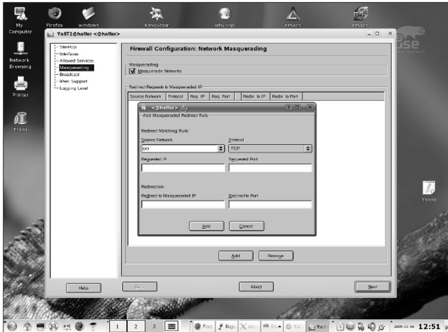
Figure 24-7: Enabling Masquerading
