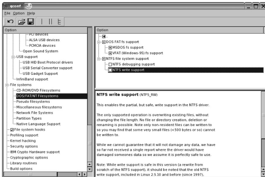
Figure 29-4: Selecting options in the xconfig interface
