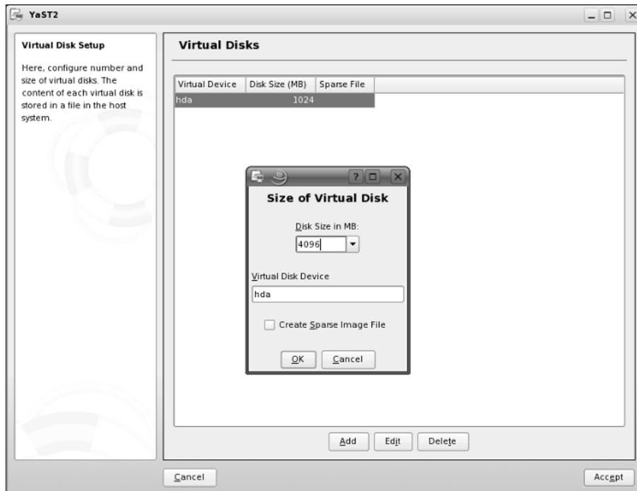
**Figure 28-9:** Setting Xen disk image options in YaST
