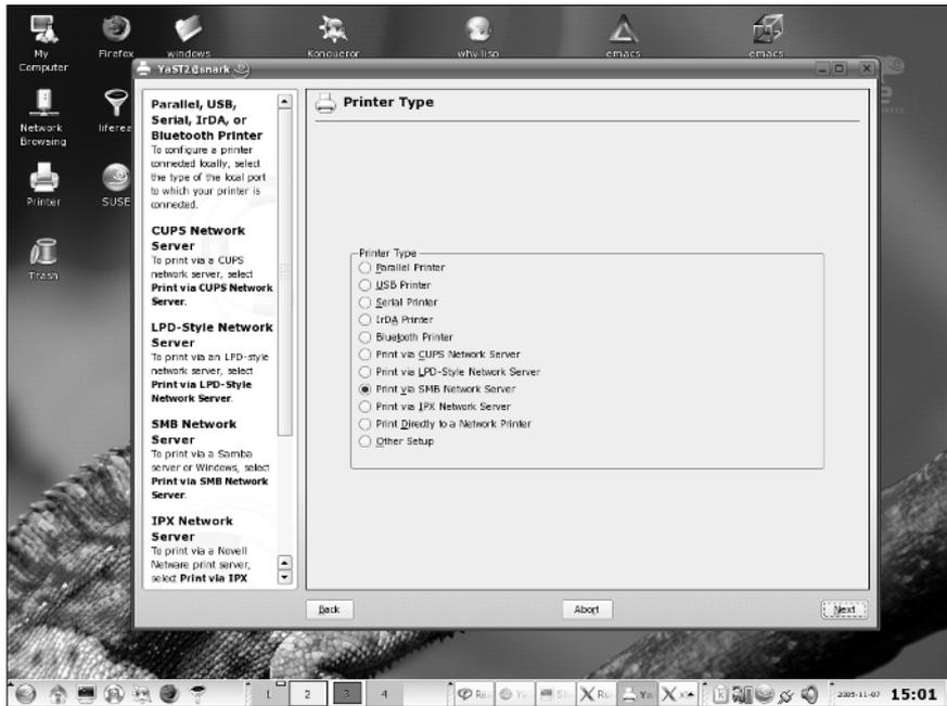
Figure 18-9: Specifying the printer type in YaST
