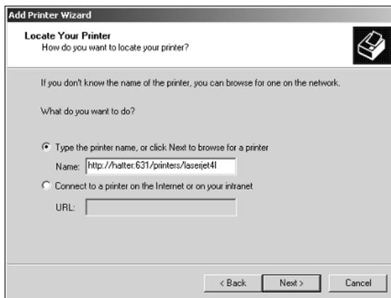
**Figure 19-7:** Setting up printing to a remote CUPS server in Windows
