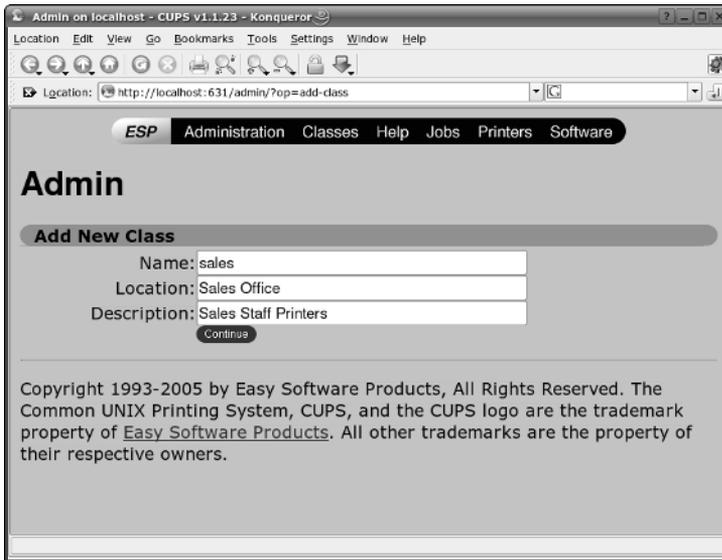
**Figure 19-10:** Adding a class in the CUPS web interface
