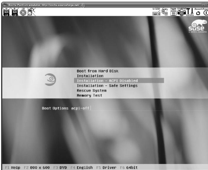
Figure 28-4: Starting a SUSE installation in `bochs`
