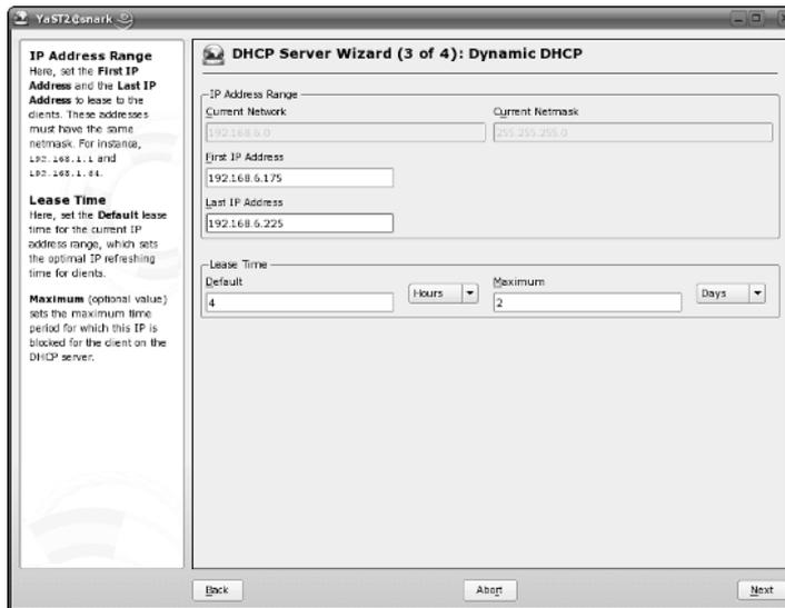
**Figure 20-3:** The Dynamic DHCP Screen in the YaST DHCP Server Wizard
