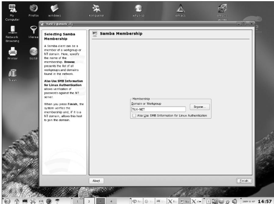
Figure 18-4: Samba Client configuration pane in YaST
