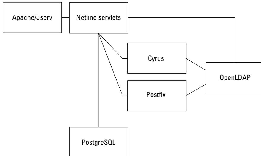
**Figure 30-12:** Conceptual overview of SLOX components
