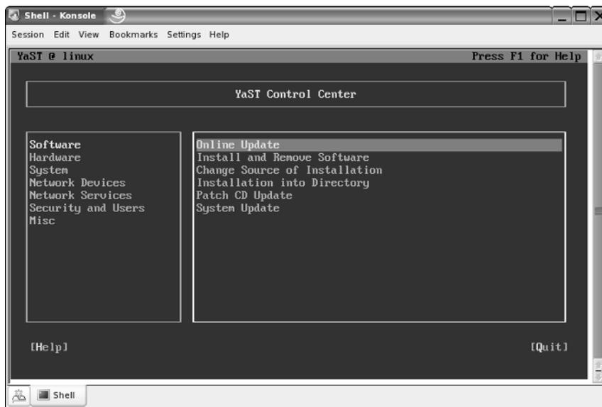
**Figure 18-21:** Main screen of the non-graphical version of YaST
