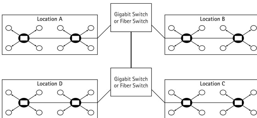
Figure 4-5: A WAN with a gigabit/fiber switched backbone
