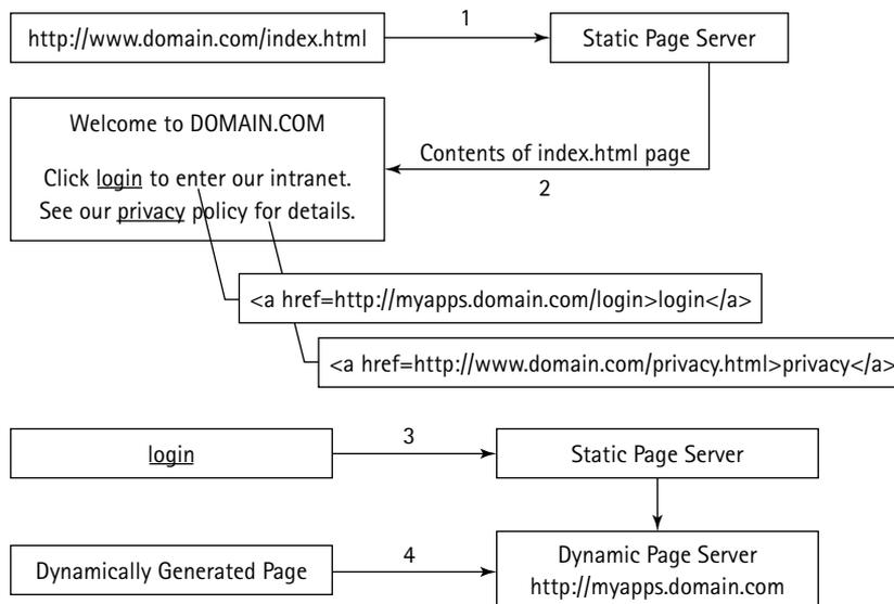
Figure 5-1: Separating static and dynamic (mod\_perl script-generated) contents
