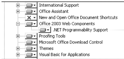
Figure 12.23 To integrate OWC with .NET applications you have to install the OWC PIAs.
