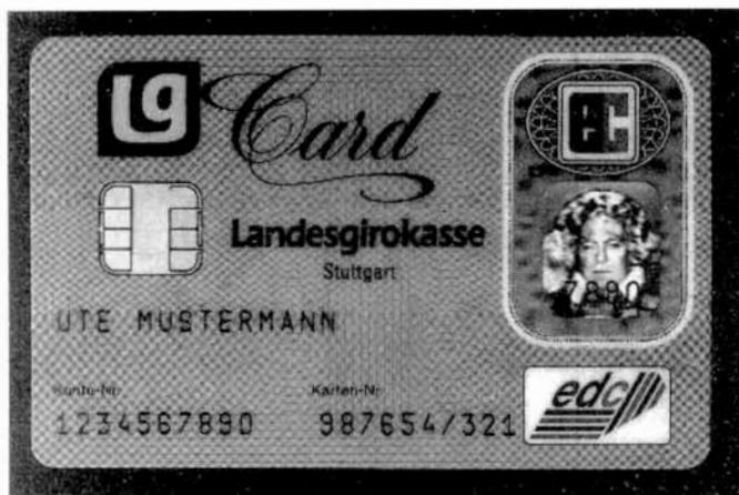
**Figure 10.2** Example of a personalized Eurocheque smart card with a microprocessor (source: Giesecke & Devrient)
