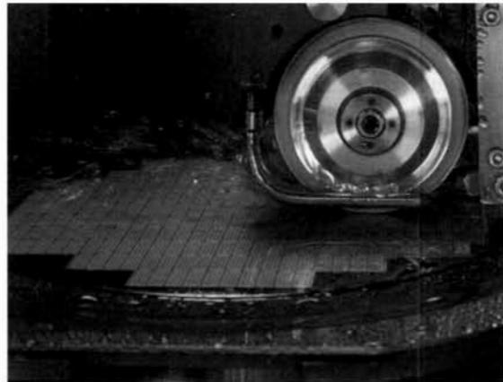
**Figure 5.19** Sawing plate of a wafer with water cooling (source: DISCO)
