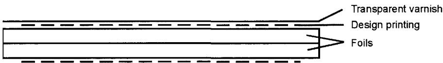
**Figure 3.10** Structure of a two-layer card with external printing and protective varnish
