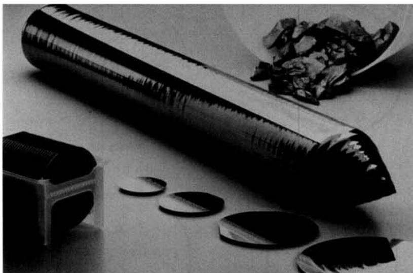
**Figure 5.11** From the top right: polycrystalline parts, single crystal, polished wafer in different sizes, wafer in transport containers (source: Infineon)
