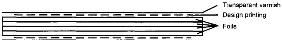
Figure 3.13 Structure of a four-layer card with external printing and protecting varnish
